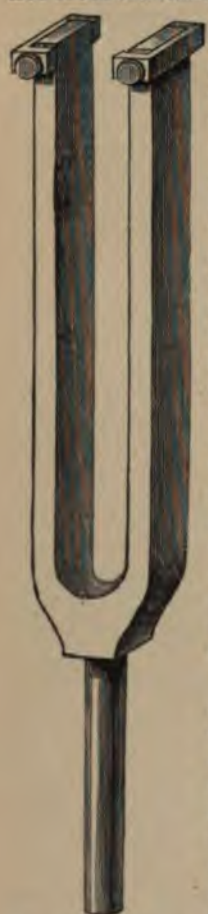
FIG. 1.—Heavy Prismatic Tuning Fork, with Movable Clamps. (Half natural size.)
